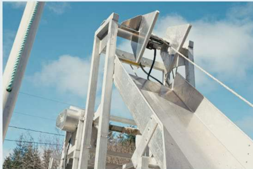
The cultivation line is hydraulically pulled up to the top of the chute and then automatically separated from the line by a mechanized cutting device.
