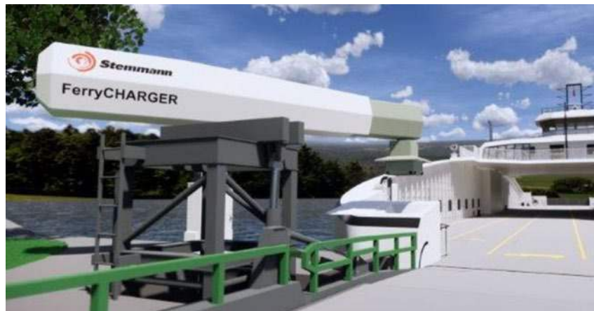
Figure 5: Stemann-Technik Third Generation Crane Based RCS
